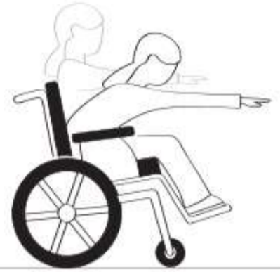
Figure 5.7: Forward reach in wheelchair
